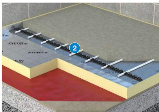
Thin-R Underfloor provides an efficient means of floor insulation. It has the strength and thermal properties required to reach the high performance U-Values asked for in the Building Regulations.
