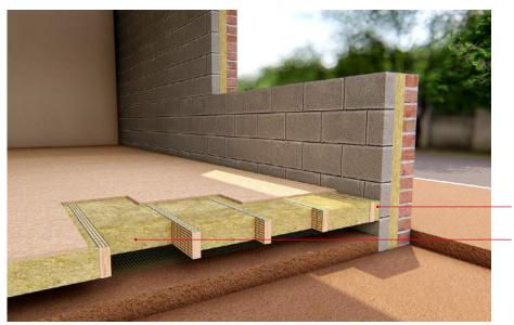
Perimeter edge insulation between joist and wall
